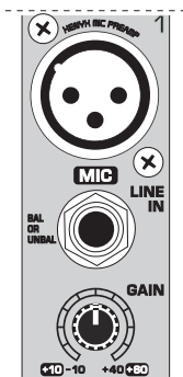
Fig. 2.1: Connectors and controls of mic/line inputs
