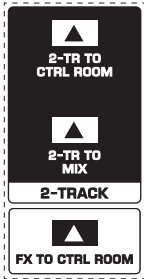
Fig. 2.12: Assignment switches of the main section
