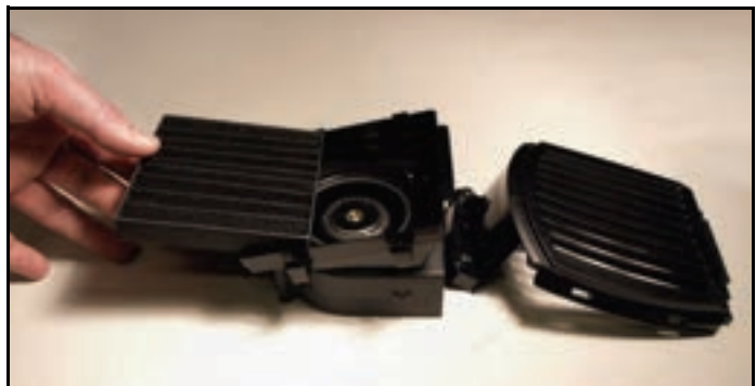
Figure 15: Head air filter alignment
