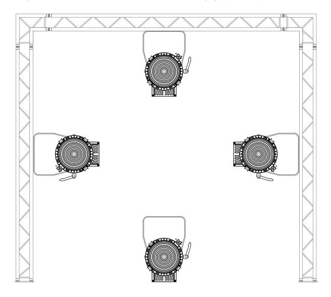
The Elumen8 Virtuoso 2000 Fresnel WW can be operated in a number of mounting positions as shown in the diagram above, hanging upside-down from the ceiling or truss, mounting sideways on truss or stood upright on a flat level surface. Always use a safety wire as an extra safety precaution to prevent damage/injury in the event a clamp fails (see the next page for clamp installation). Never use the carry handles for secondary attachments.
